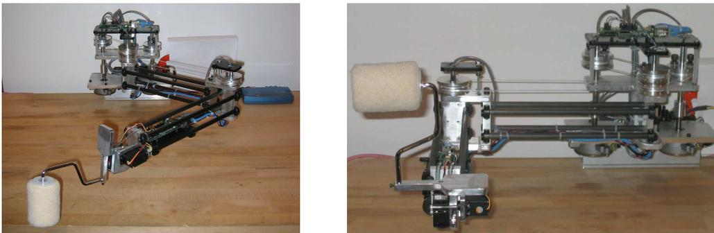
Figure 4-10: Proof-of-Concept 3 – Four degree of freedom arm with drive-system compliance, a hierarchical control architecture, and a servo-mounted paint roller. **Left:** Front angle view. **Right:** Front view.
